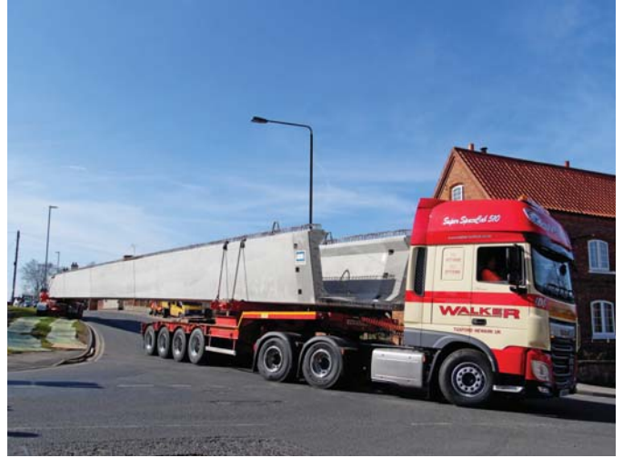
Above: Transporting the nine 42m-long, 90-tonne beams was a major logistical operation that required the co-operation of highway authorities along the route.
